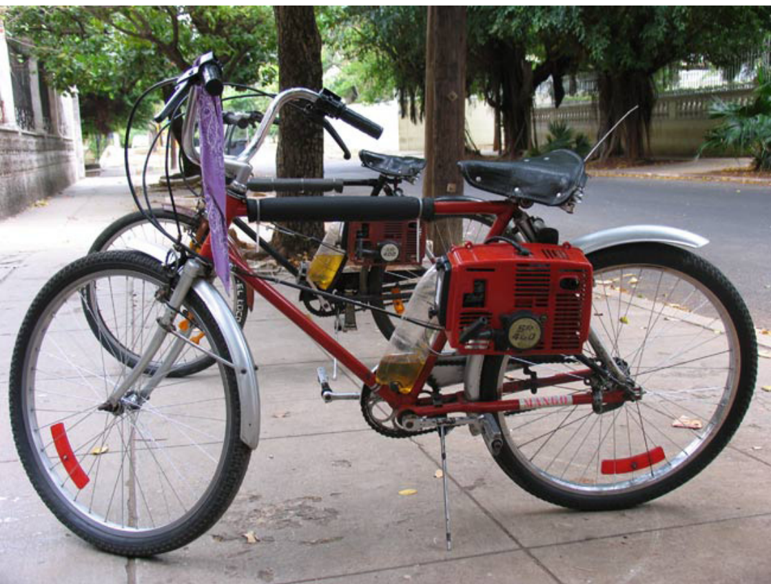
Fig. 05 - Ernesto Oroza, Technological Disobedience Device , Rikimbili, 2007. Bicycle + gasoline pump water, fumigation devices or gasoline engines chain saw. For more Rikimbilis, go to: < http://www.ernestooroza.com/rikimbili/ >. © Ernesto Oroza.
